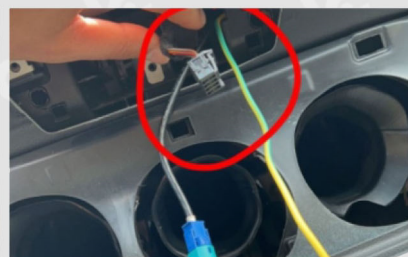
15. Leave this plug aside, no need plug. (it is for original Screen power)
