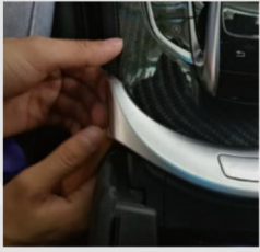
1. Use Trim removal tool to pry up central armrest compartment silver trim.
