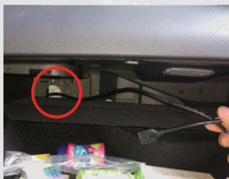
13. Snake Android USB cable to Glove box
