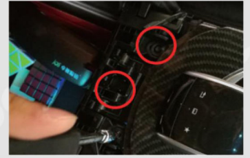
2. Remove two screws holding the armrest
