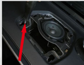
6. Remove the screws holding the screen
