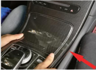
3. Carefully pull up on the center console panel slowly.
