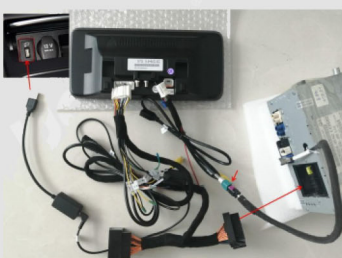
17. Plug USB audio box to 3.5mm male cable and plug in car AUX USB
