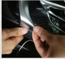
1. Use Trim removal tool to pry up central armrest compartment silver trim.
