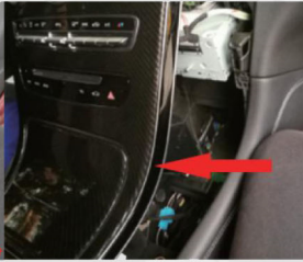
3. Carefully pull up on the center console panel slowly.
