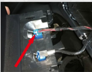
9. Unplug cables behind monitor
