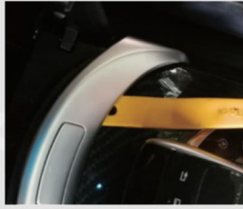
1. Use Trim removal tool to pry up central armrest compartment silver trim.
