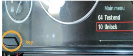
4. Add the last 5 digits of the chassis number (for example, as shown in the left figure  $5+1+9+0+6=21$ ), fill in the number 21 in the CODE position, and then press the key to exit;
